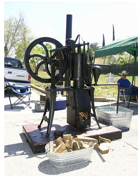
A typical late nineteenth/early twentieth century water pumping engine by the Rider-Ericsson Engine Company
